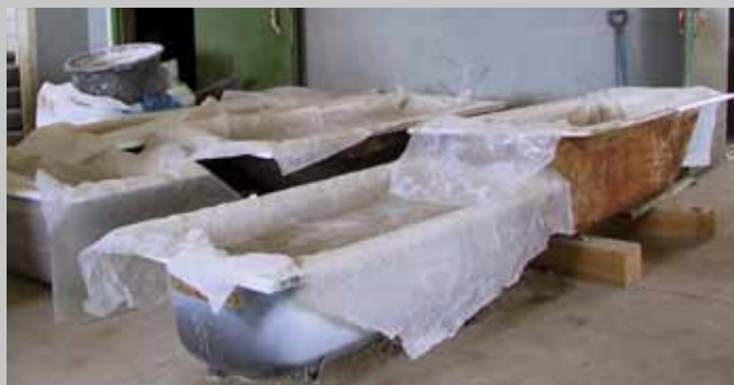
Lime mortars maturing in tubs. Before use, the mortars were allowed to mature for a couple of months during which they were mixed weekly.
