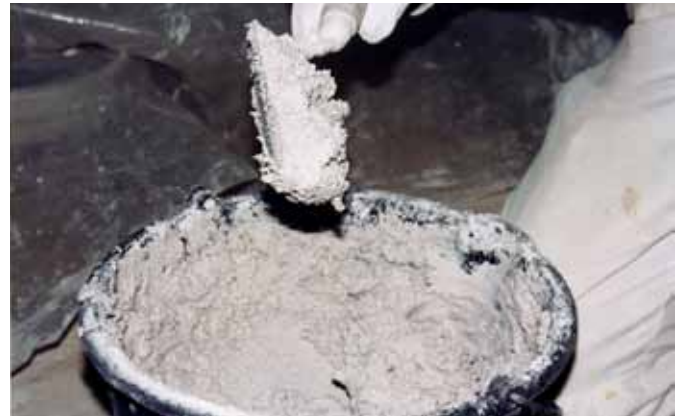
This mortar has cured long enough and the mason has worked it well before use. A mortar must be stiff enough to cling to an inverted trowel or shovel and slide off when turned sideways.
