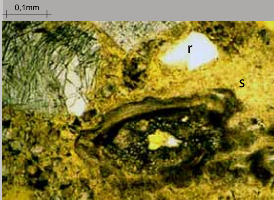
Old lime mortar with hydraulic components. A reaction border has formed around the mineral in the middle. The section shows lots of binder and only one aggregate granule. Photomicrograph \times 20 , parallel nicol (//-nicol).
