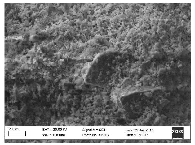
Figure 6: Scanning electron microscope (SEM) image showing microporous nature of binder and intimacy of bond with aggregate in historic lime mortar. Kilmahew Castle, Strathclyde c.1500-1700. Quartz aggregate, binder is calcite rich. Note the scale bar and size of the pores ca.  $1\mu$ m (Wiggins 2015).
