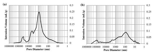
Figure 7: Pore size distributions of (a) historic lime mortar from Balvenie Castle; (b) modern NHL-based lime mortar in use at Urquhart Castle after 2-yrs field curing. Note the distinct discord in predominant pore size in addition to the discord in overall porosity (the area under the curve) (Wiggins 2015).
