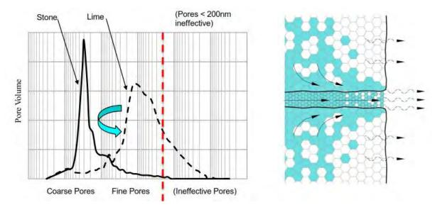
Figure 2: Poultice mechanics (log scale) and as applied to a 2-D cross-section through a mortar bed joint with inferred water movement pattern (salt advection) (Wiggins 2015).
