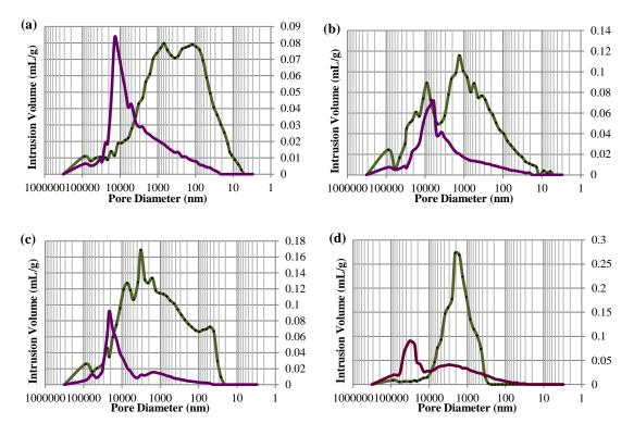
Figure 4: Data pore size distributions of sandstone and lime mortar. (a) Bothwell Castle, South Lanarkshire; (b) Melrose Abbey, Roxburghshire; (c) Newark Castle, Port Glasgow; (d) Saltmarket Tenements, Glasgow. The purple line represents stone, the green line represents lime mortar (Wiggins 2015).
