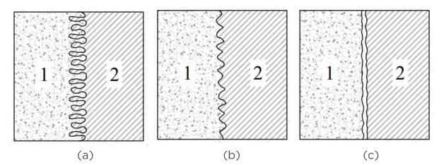
Figure 5: Theoretical variations of bond intimacy and their effect on capillary flow. From left to right: (a) represents hydraulic continuity; (b) represents natural contact; (c) represents an air space formed by shearing of the interface manifesting in interruption to fluid phase movement (Wiggins 2015).
