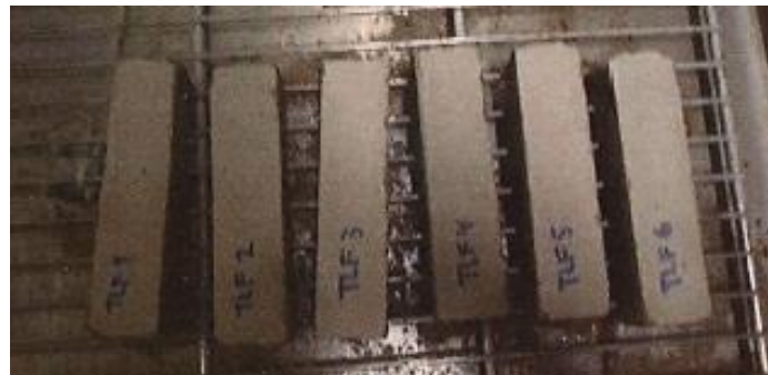
The Turku Castle mortar LLh 15/85/440 + air-entrainment agent, after 100 freezing cycles
