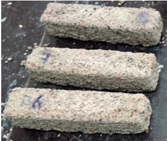
The Olavinlinna reference mortar LLh 15/85/525, after 50 freezing cycles
