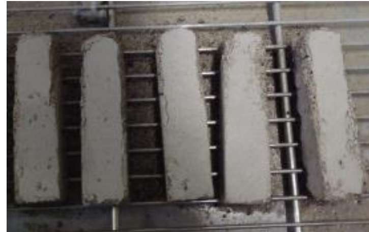
The Turku Castle mortar LLh 15/85/525 + air-entrainment agent, after 25 freezing cycles
