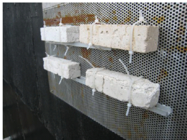
Fig. 6 Test samples was mounted on the south wall to test the resistance to weathering
